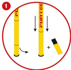
**1** Each post is assembled from three pieces. The section with the FUNTEC sticker is the middle piece. The bottom section consists of a larger and smaller section. You can remove the short section of the post if required to reduce the net height to the recommended ladies height.
