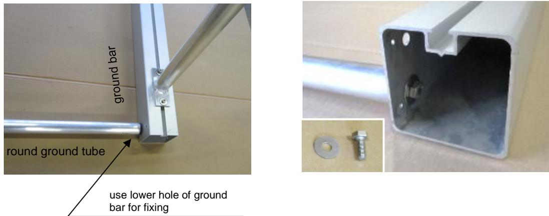
Stick caps in the open ends of ground bars. Bore them with drill 1.5 mm through the holes provided in the ground bars. Then fix plug pins with a hammer/mallet (see the following pictures). Tighten again all screws fixed at the net hoops.
