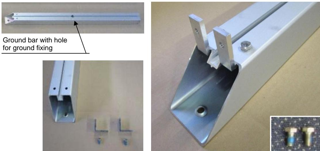
Now turn ground spars and insert from the inside 1 wide angle (without treaded hole) in each ground bar (see picture bottom left). Stick from the outside 1 hexagon socket screw M 8 x 20mm each through holes of ground bar and connection angle. Add spring washers A8, DIN 127, screw nuts M8, DIN 934 and tighten them (see mid picture). Adjust angle parallel to the outside edge of the ground bar (see picture bottom right).
