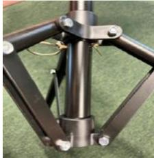
Step 2: Slide the basket #2 onto the base and open up the basket. After that lock it with pin #4.
