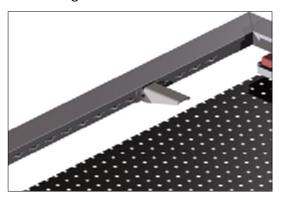
The metal angles shown on the left serve as a stilt for the screwed screen printing boards. The accordingly equipped frame profiles have to be mounted with the closed side of the angle pointing upwards.
